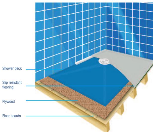
The Premier Shower Deck can be installed into an existing timber floor by removing the floorboards and fixing the former directly onto the joists. If the deck protrudes more than 100mm over a joist, support noggins should be installed. The floor should be brought level with the former to make the room level and ready for a suitable floor covering.
